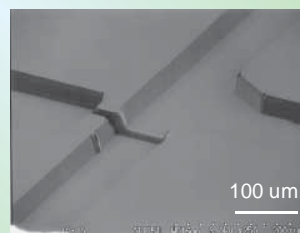
SEM picture of prominent structure and air vent
